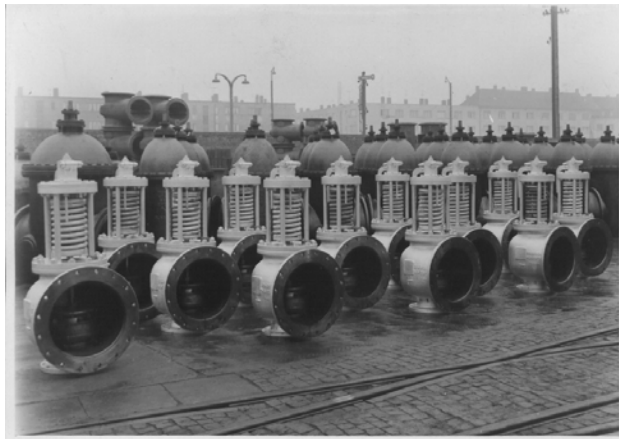
1958: Si 61 Full lift safety valves, supplied to protect a plant for utilizing geothermal steam
